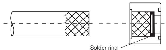
Apply heat by moving the flame round and heat the mass of the fitting rather than the tube.
